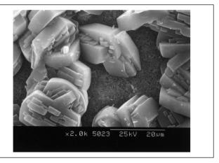
Figure 7. SEM surface of the membrane prepared on unseeded  $\alpha$ -Al<sub>2</sub>O<sub>3</sub> tube with 0.1  $\mu$ m pore size at 175°C for 24 h using colloidal silica.
